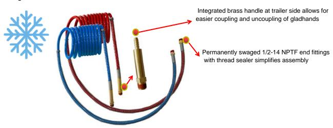
Applications: Connect the tractor and Trailer hook up (Long lead end to tractor and short lead end to trailer)
